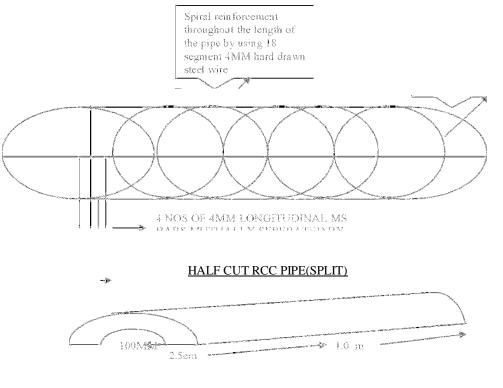
18 NOS OF SEMICIRCULAR REINFORCEMENT BY USING 12 GAUGE (2.4MM HARD DRAWN STEEL WIRE PLACED EQUIDISTANTELY THROUGHOUT THE LENGTH O THE PIPE
